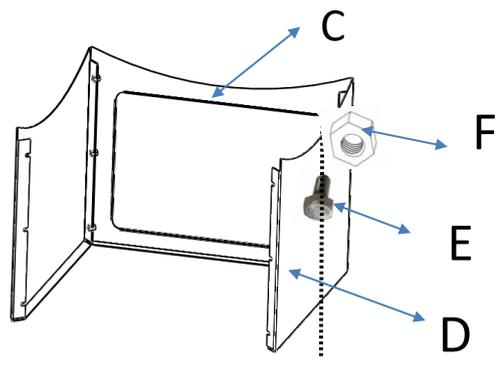
Connect the left panel(D) and rear panel(C) with 3pcs screws(E) and 3pcs nuts (F)
