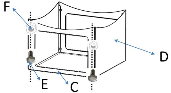
Connect the front panel (C) and left, right panel (D) with 6pcs screws (E) and 6pcs nuts (F)
