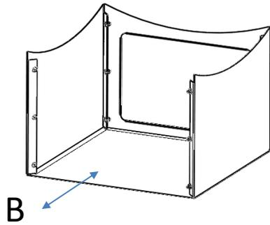
Insert the bottom panel (B) in the left, right, rear panel
